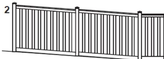
**2 SLOPING METHOD:** This fence follows the grade or slope with the rails parallel to the ground. Taller posts are not required but the horizontal post spacing may need to be reduced to avoid rails being too short. Miter-cut rails to fit grade. On extreme slopes, pickets may require cutting.
