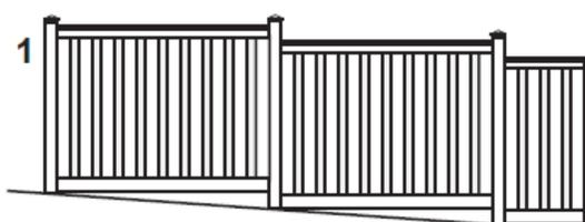
**1 STEP METHOD:** This fence gradually "steps" down the slope so each section is the same length and the rails remain level. Gaps will exist under the fence. The downhill post will need to be set higher to allow attachment of the top rail. Taller posts may be required. When laying out the fence spacing between posts, the distance must be measured horizontally and not parallel to the ground.
