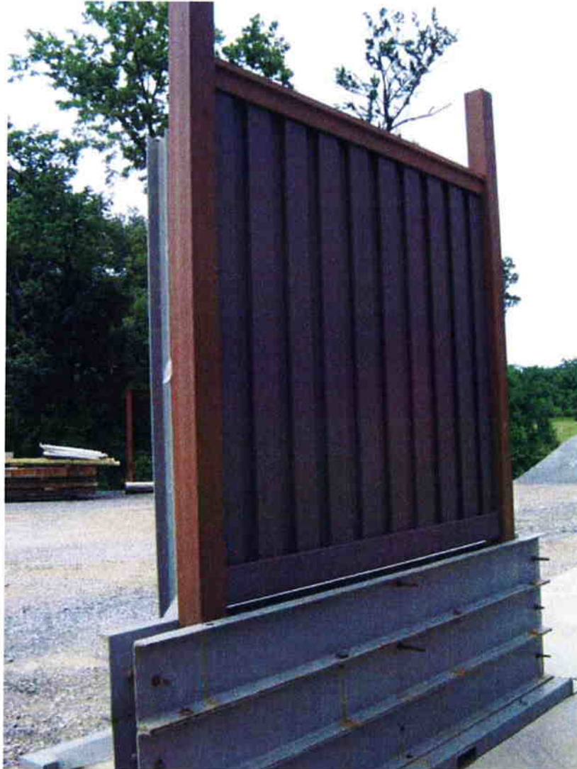
Photo No. 1 Seclusions TM Privacy Fence as Installed in Rigid Test Fixture
