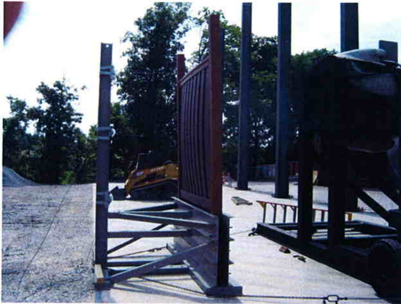
Photo No. 2 Typical Test Setup (Test Fixture and Wind Generator)
